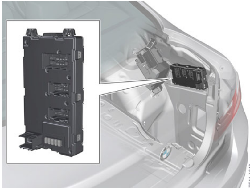
F30 REM installation location
